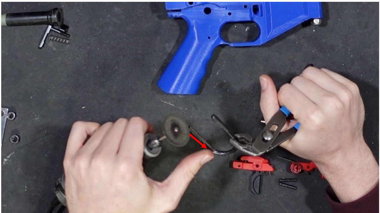
Using a pair of pliers to hold the U-bolt, a Dremel with a cutoff wheel makes short work of the modification to the legs.
