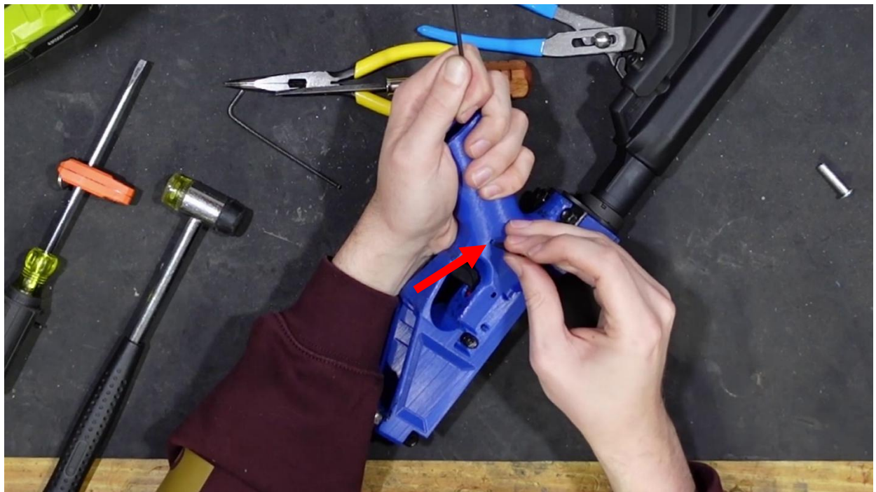
While keeping it compressed, stick your 1/8" roll pin (or 3mm pin, or whatever hardware you plan on using) into the cross hole.
