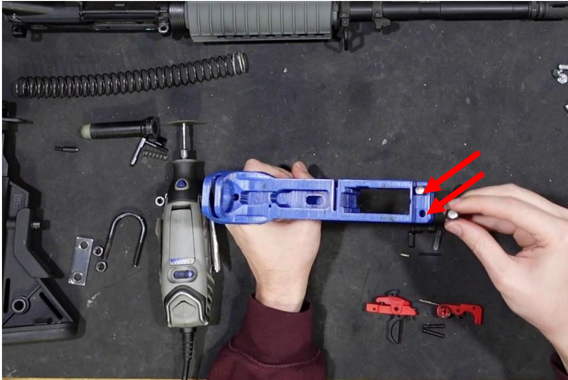
Install the eyebolts into the front holes
