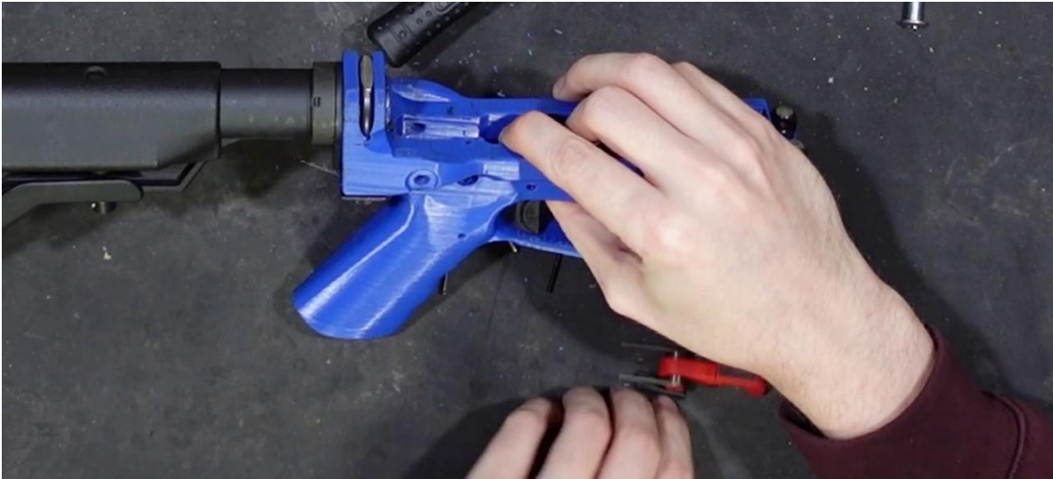
Install the trigger and disconnecter – this process is just like on a standard AR15.
