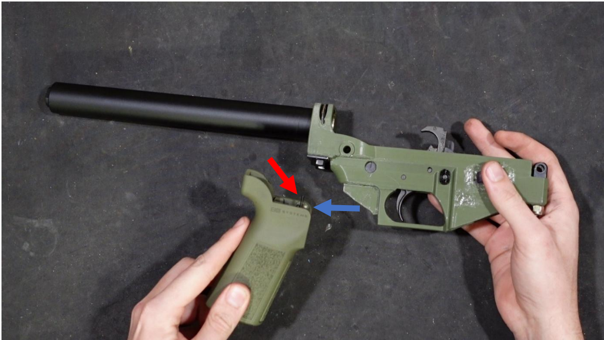
With the spring and screw inserted into the pistol grip, mate the grip up with the lower.
