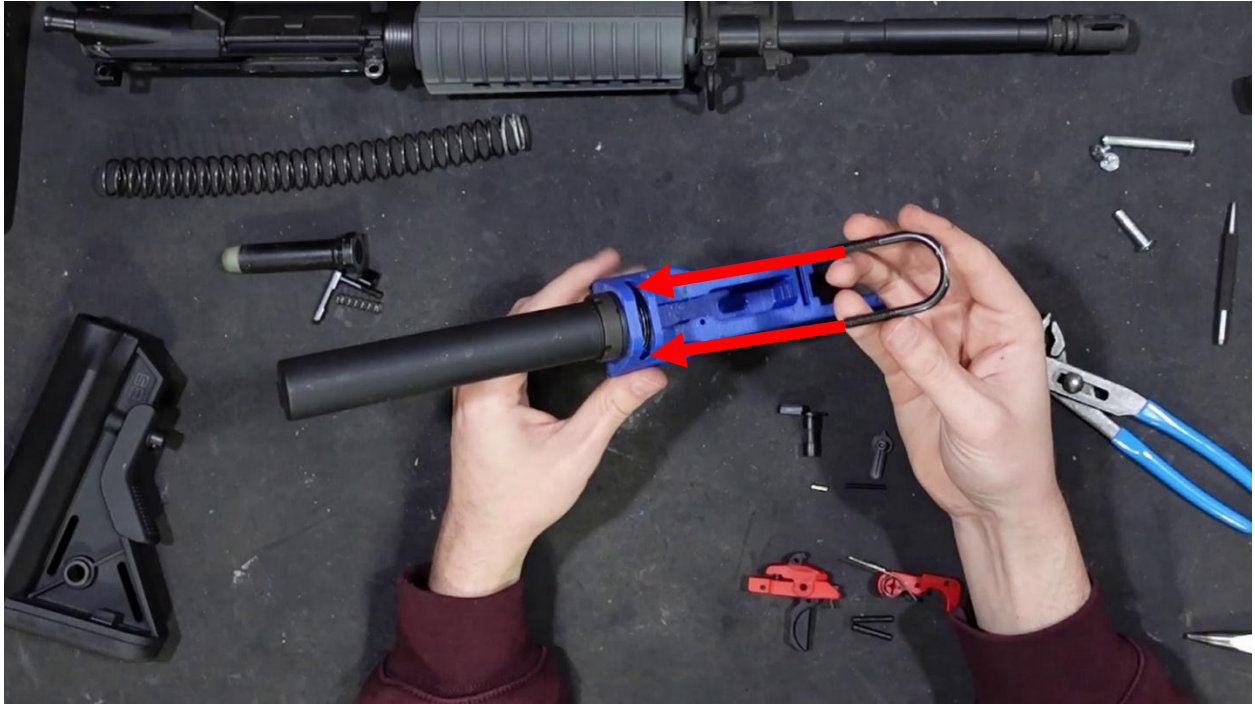
Place the u-bolt down onto the tube
