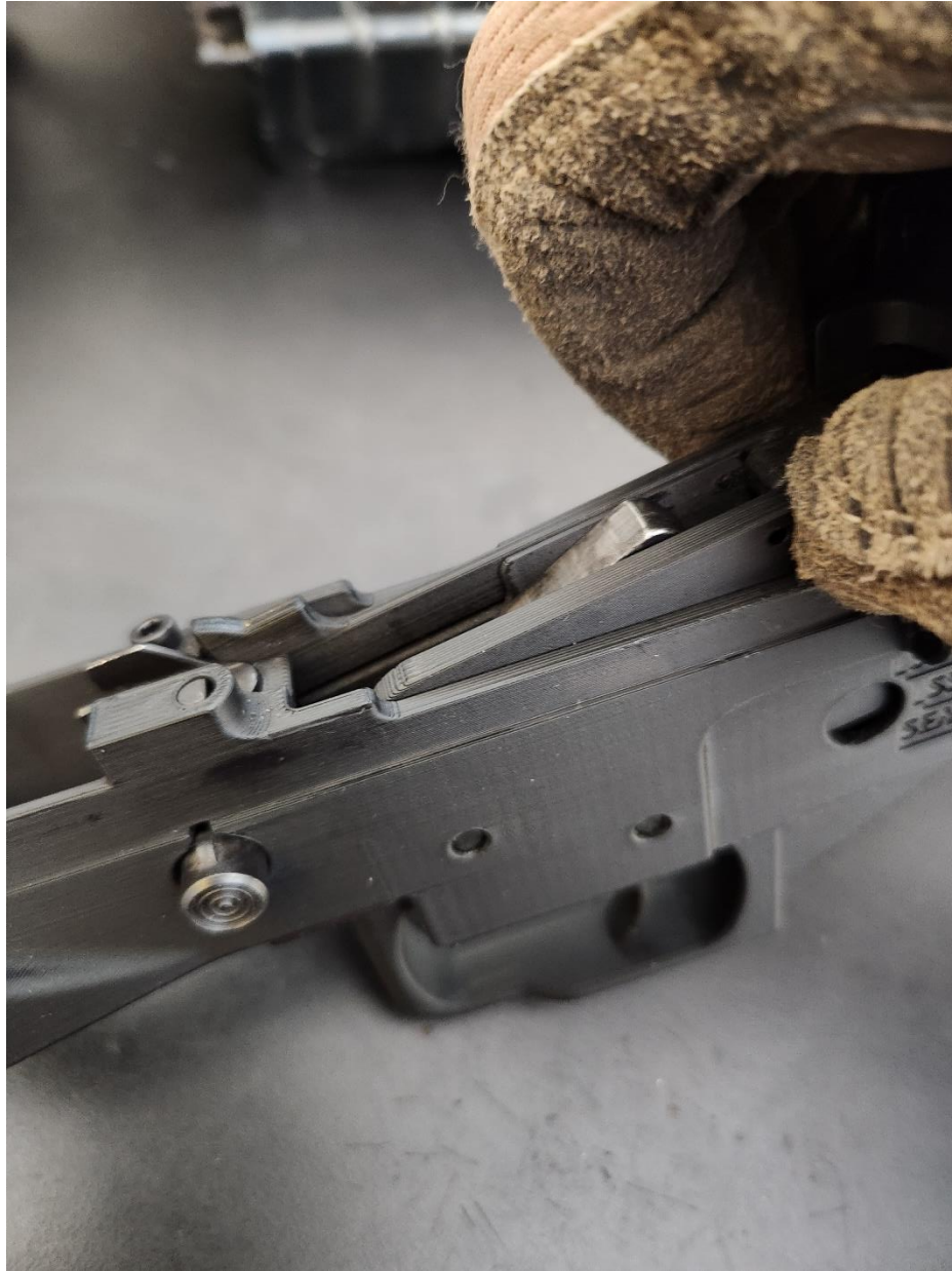
Figure 3: Installing Housing into Lower
