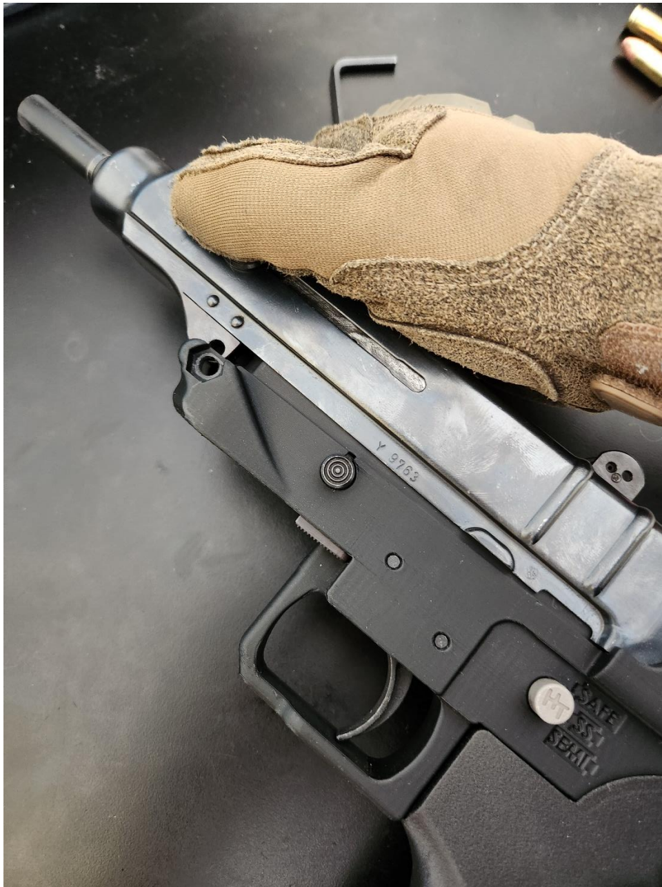
Figure 5: Installing Upper Receiver onto Lower
