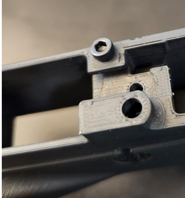
Figure 1: Reinforcement Screw Installed
