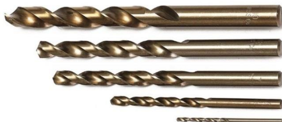
2mm, 4mm, 7mm and 10mm standard length DIN 338 high quality HSS-CO (5% cobalt) drills.
