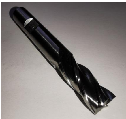
1X - DIN 844 (DIN 844K) standard length 10mm end mill with four cutters.
