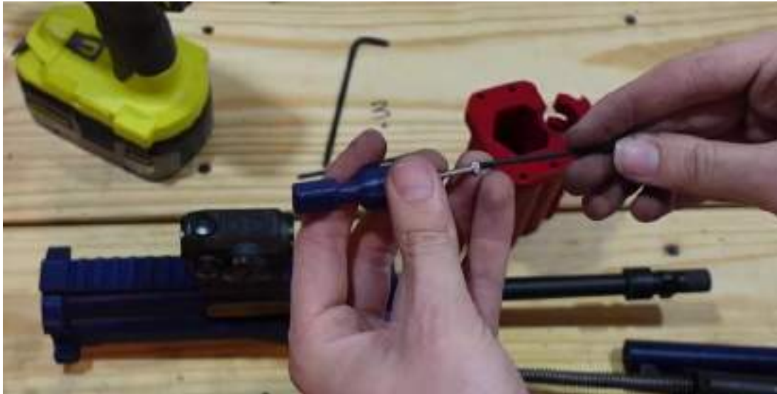
Screw the M3 bolt into the center recess on the charging handle.
