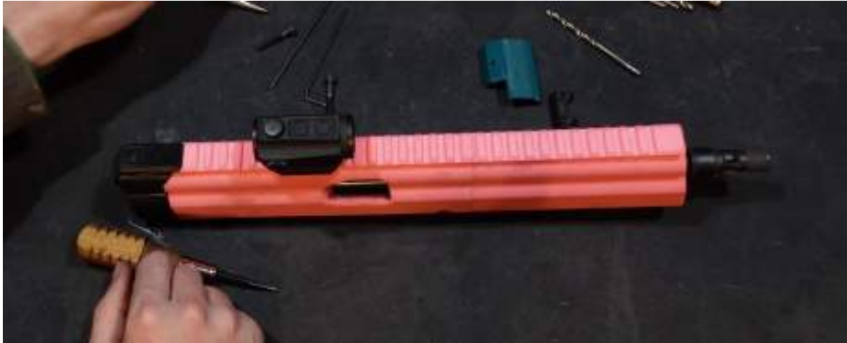
The nut cover is installed by simply pushing it onto the endcap.
