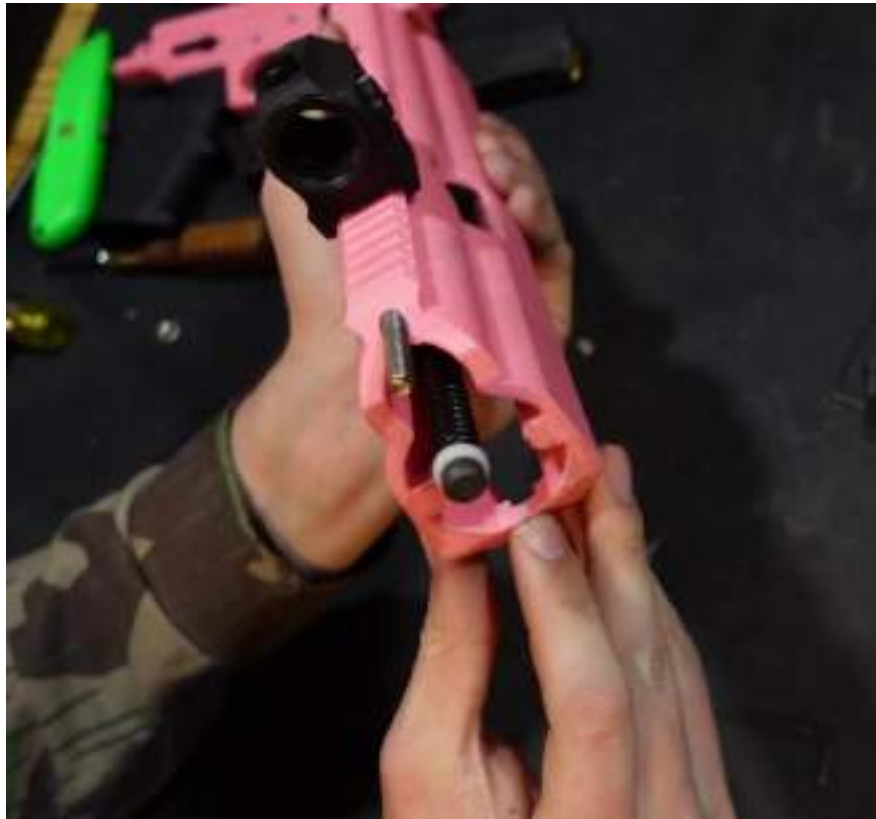
The recess for the nut in a k-length upper. For the full-size uppers, this recess will contain the nut, but for the short uppers, you will have to hold it in place.
