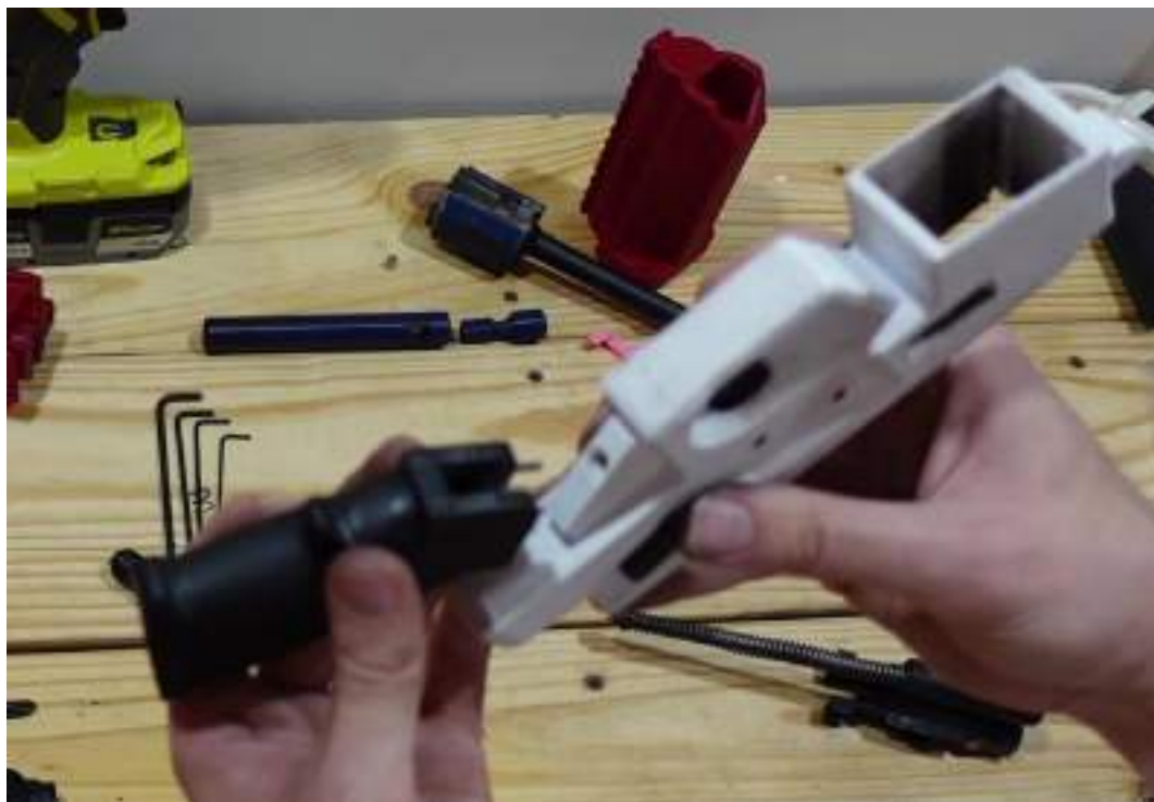
Install the pistol grip and detent spring
