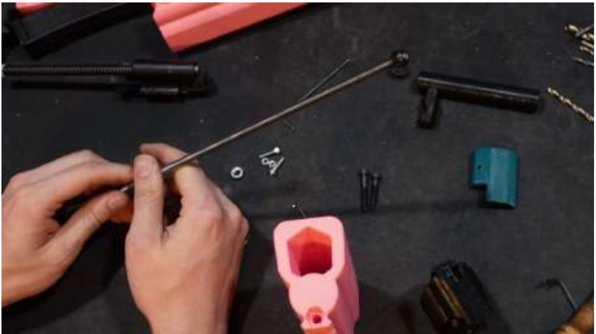
Thread the locking nut on until it is flush with the end of the rod.
