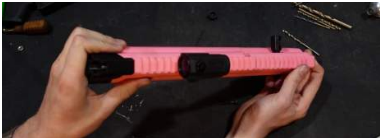
Push the endcap onto the threaded rod.
