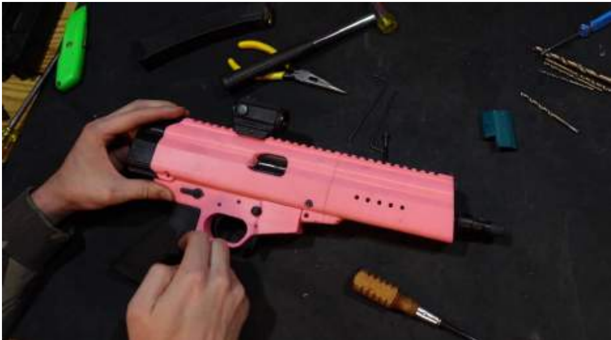
Finally, take your lower receiver and mate it up with the upper receiver. You will use two M5x35 or M5x30 bolts to secure the lower to the upper. The M5x35mm option allows you to put a nut on the end of the bolt to retain it in a more secure manner to the upper. These bolts should have a little resistance when installing them, but shouldn't take hard hits.
